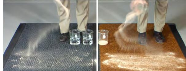
**STEP 1** - 1 cup of sand is poured on the Waterhog™ 3' x 5' mat and a cup of sand is poured on a finishing/rental 3' x 5' mat
